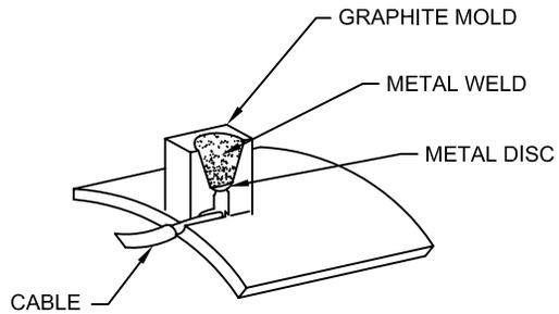
3) HOLD MOLD FIRMLY WITH OPENING AWAY FROM OPERATOR, IGNITE WITH FLINT GUN
