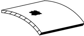
4) REMOVE SLAG FROM CONNECTION, COVER CONNECTION WITH COMPATIBLE COATING AND CAP OVER ALL EXPOSED METAL
