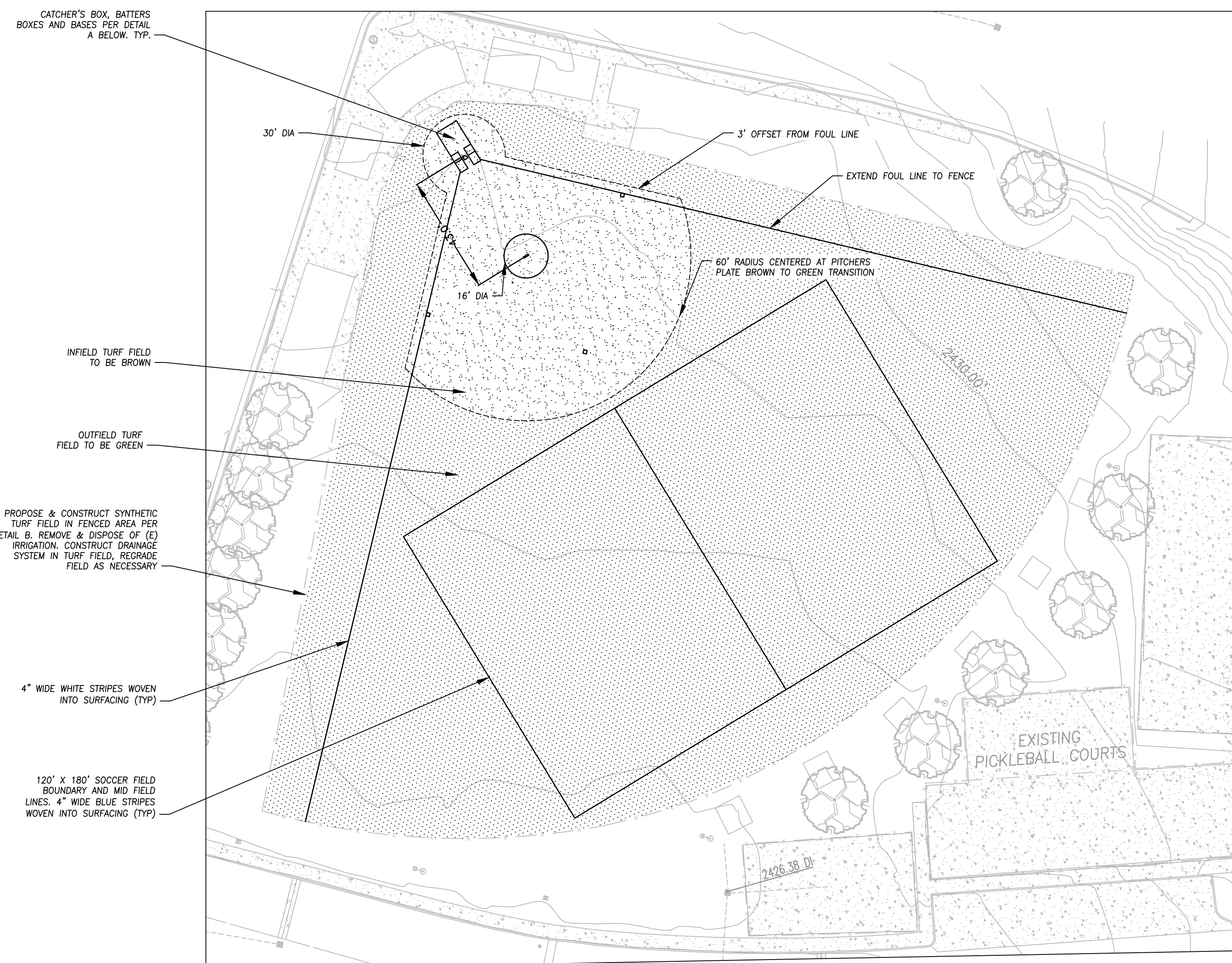
SOFTBALL FIELD ARTIFICIAL TURF CONSTRUCTION PLAN
