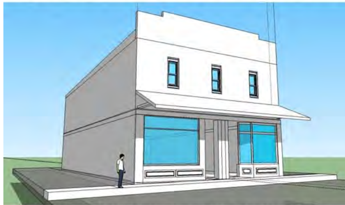
Shed Awning – Made of lighter materials using posts or braces
