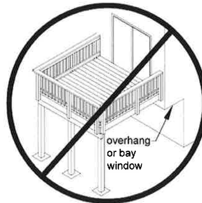
Figure 18. No Attachment to House Overhang with Ledger.
