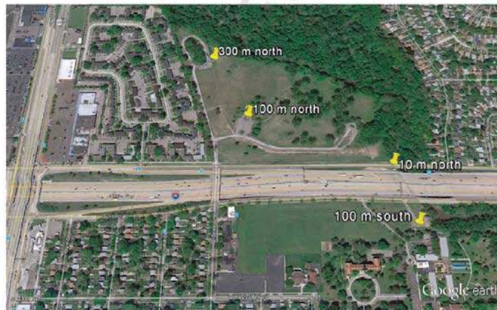
Fig. 1. Monitoring site transect array across I-96 west of Detroit established for the EPA/FHWA National Near Road Study and used as a component of the NEXUS study. I-96 runs east-west and Telegraph Road is the multi lane road running north-south to the west of the sampling sites.
