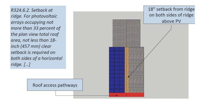
R324.6.2.1. Alternative setback at ridge. Where an automatic sprinkler system is installed within the dwelling in accordance with NFPA 13D or Section P2904, setbacks at ridges shall conform with one of the following:
