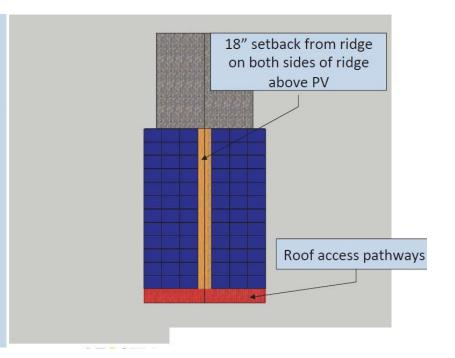
R324.6.2.1. Alternative setback at ridge. Where an automatic sprinkler system is installed within the dwelling in accordance with NFPA 13D or Section P2904, setbacks at ridges shall conform with one of the following:
